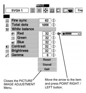
NOTE : The Fine sync and the Total dots cannot be adjusted when "RGB," "HDTV1035i" or "HDTV1080i" is selected on the SYSTEM MENU (P22 and 23).
